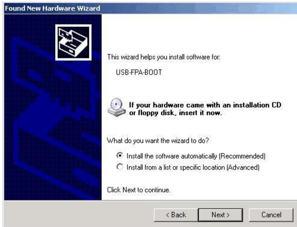
Figure 3.2: New Hardware Wizard, step 2. Select “Install the software automatically.”
