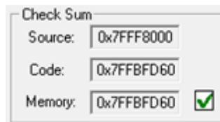
Figure 9.1: Check Sum information compared between the file and MCU memory.
