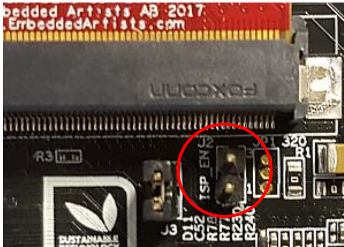
Figure 3 - J2 jumper (opened state) on a COM Carrier Board V2
