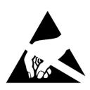
Make it a habit always to first touch the metal surface of one of the USB connectors on the OEM Base Board (which the Display Expansion Board is connected to) for a few seconds with both hands before touching any other parts of the boards. That way, you will have the same potential as the board and therefore minimize the risk for ESD.
