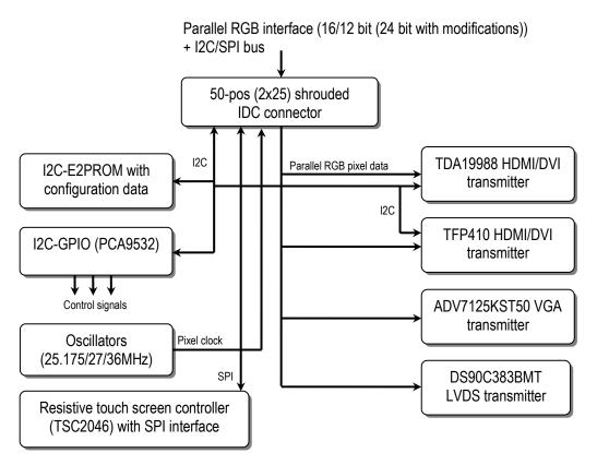
Figure 2 - The Display Expansion Board Block Diagram
