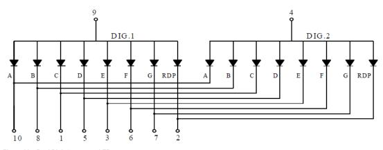
Figure 32 – Dual Digit 7-segment LED
