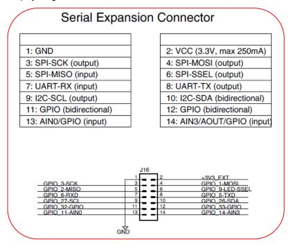
Figure 67 – Serial Expansion Connector on Schematic Page 7
