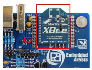
Figure 64 – XBee® Module Mounted in J15
