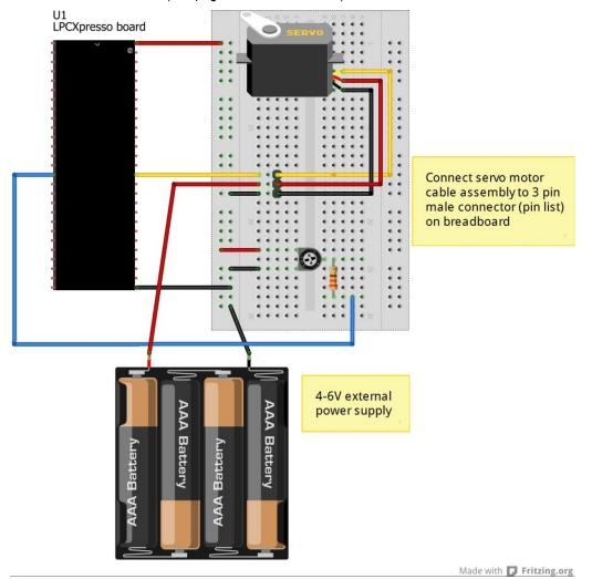
Figure 45 – Breadboard with Servo Motor
