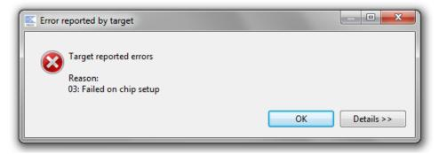
Figure 94 – LPCXpresso IDE Error: Failed on chip setup
