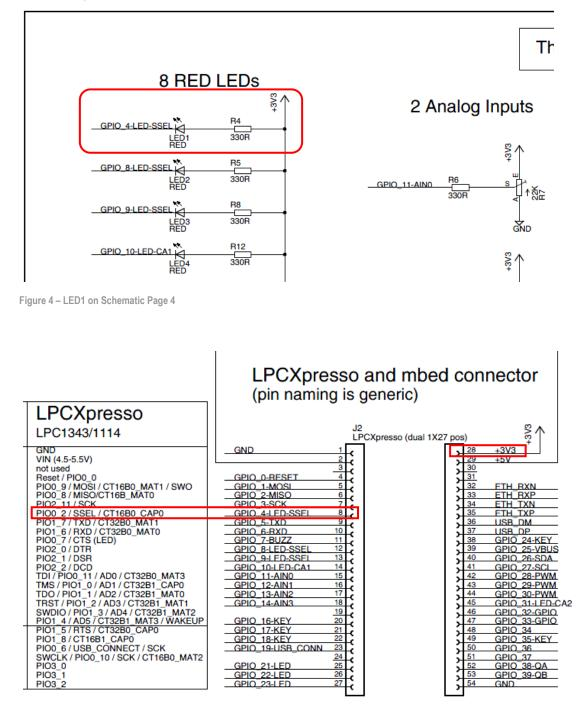
Figure 5 – Signal GPIO\_4-LED-SSEL on Schematic Page 2
