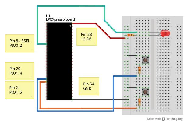
Figure 14 - Breadboard Connections for SW2, SW3 and LED
