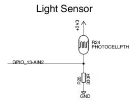
Figure 25 – Light Sensor on Schematic Page 4
