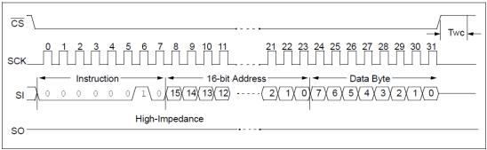
Figure 51 –25LC080 Byte Write Sequence
