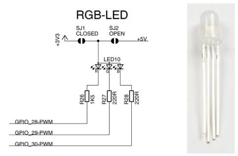
Figure 29 - RGB-LED, LED10, on Schematic Page 4
