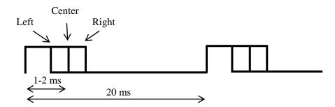
Figure 44 – PWM Signal for Servo Control
