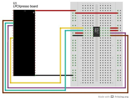
Figure 54 – Breadboard with SPI E2PROM
