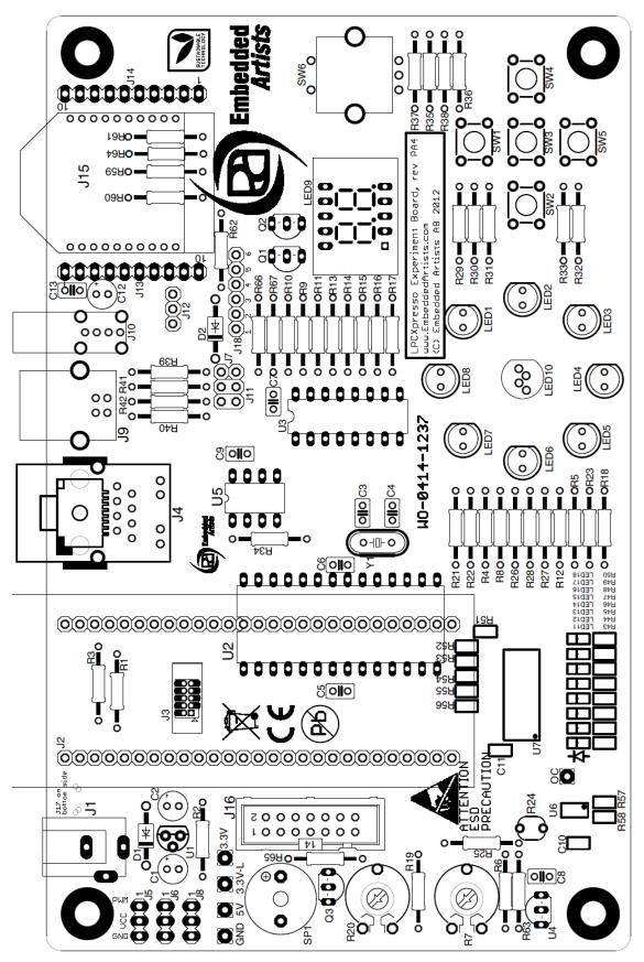
Figure 2 - LPCXpresso Experiment Kit PCB with Component Designators
