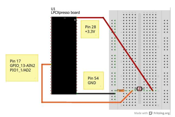
Figure 26 – Breadboard Connections for Light Sensor R24
