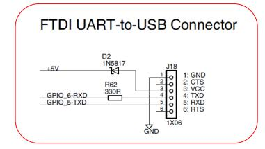
Figure 58 - J18, D2 and R62 on Schematic Page 7
