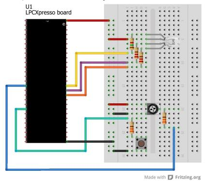
Figure 31 – Breadboard Connections for RGB-LED Experiments
