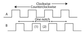
Figure 20 – Quadrature Encoder Output Signals
