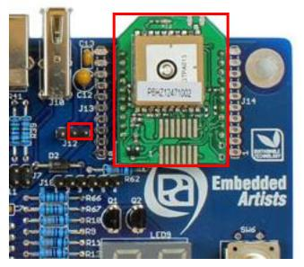
Figure 65 - GPS Module Mounted in J15
