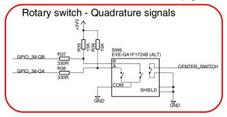
Figure 19 – Quadrature Encoder (SW6) on Schematic page 5
