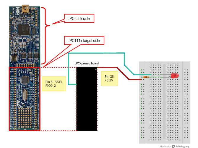
Figure 6 – Breadboard Connections for LED1 (breadboard view)
