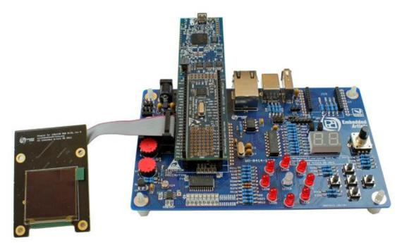
Figure 68 illustrates how the display is connected to the LPCXpresso Experiment board via a 14-pos cable.
