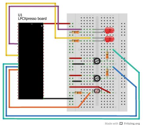
Figure 27 – Breadboard Connections for PWM Experiments
