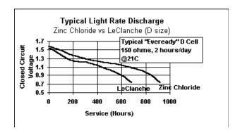
As the drain is increased, the service difference between Alkaline and Zinc Chloride. systems increases. This relationship is shown by the following discharge curves. Typical carbon zinc moderate drain is defined as a current that would discharge the cell within 10-50 hours of use at room temperature.
