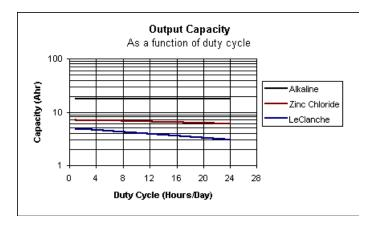
The electrochemical inputs of cylindrical D size batteries typically are in a ratio of 2:3:5 for, Zinc Chloride and Alkaline respectively. The differences in efficiency and rate sensitivity between the two systems cause variations in actual output in simulated typical applications as shown in the following table and graph:
