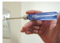
Circuit testing handle (AC80~250V/DC100~300V)
