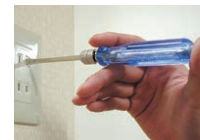
Circuit testing handle (AC80~250V/DC100~300V)
