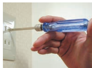
Circuit testing handle (AC80~250V/DC100~300V)
