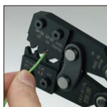
② Insert wire into barrel of contact.
