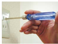
Circuit testing handle (AC80~300V/DC100~250V)
