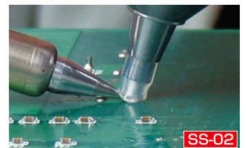
Elastic and heat-resistant nozzle can stick to soldering iron on board closely and suck up solder powerfully with less residue.
