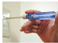
Circuit testing handle (AC80~300V/DC100~250V)
