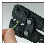
② Insert wire into barrel of contact.
