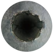
Heavily damaged or failure with the 1st Bit.
