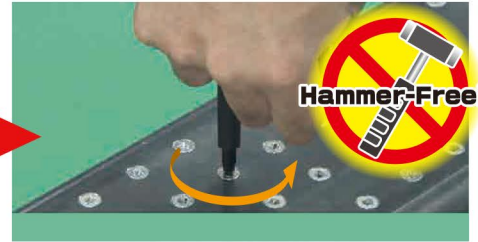
Give a jerk counterclockwise while pressing downward.
