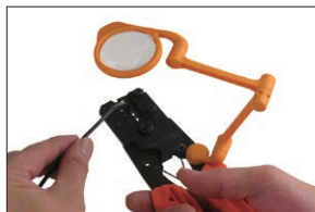
Attachment to a crimp tool
