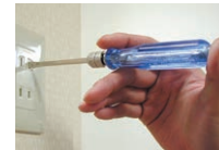
Circuit testing handle (AC80~250V/DC100~300V)
