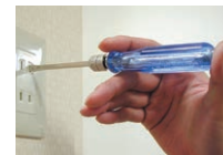
Circuit testing handle (AC80~250V/DC100~300V)
