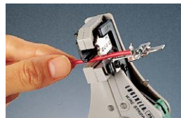
1. Insert wire into the hole applicable.
