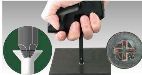
Scrape away burs in the screw recess.
