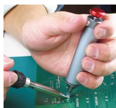
Plunger is within easy reach of thumb. It is ideal for one-hand operation in continuous work.
