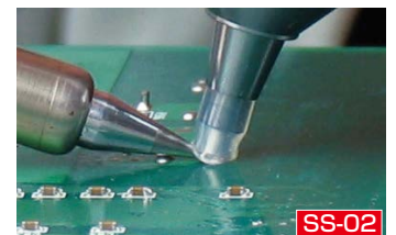
Elastic and heat-resistant nozzle can stick to soldering iron on board closely and suck up solder powerfully with less residue.
