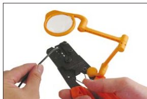
Attachment to a crimp tool
