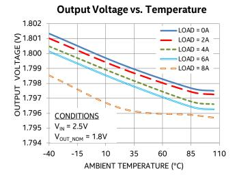
Output Voltage vs. Temperature
