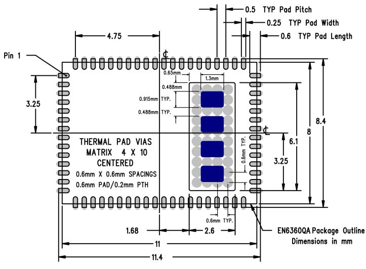
Figure 12: EN6360QA PCB Footprint (Top View)
