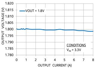
Output Voltage vs. Output Current
