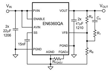
**Figure 1: Simplified Applications Circuit**
