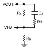
Figure 6: External Feedback/Compensation Network
