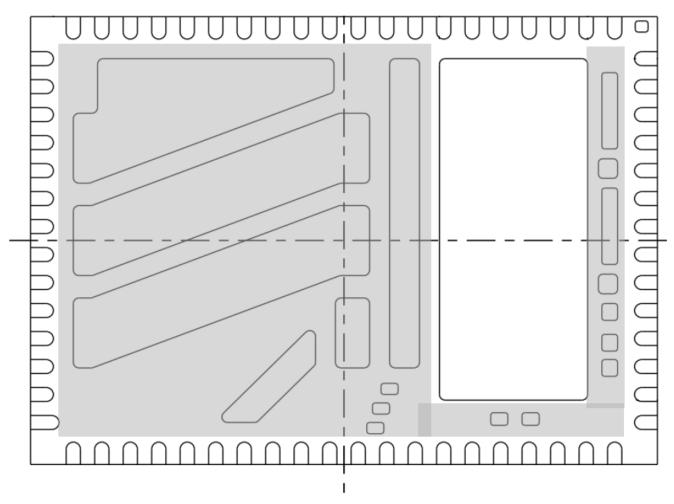
Figure 11: Lead-Frame exposed metal (Bottom View)
