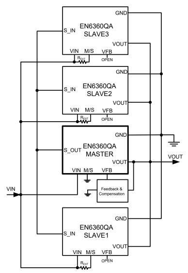
Figure 5: Master/Slave Parallel Operation Diagram POK Operation
