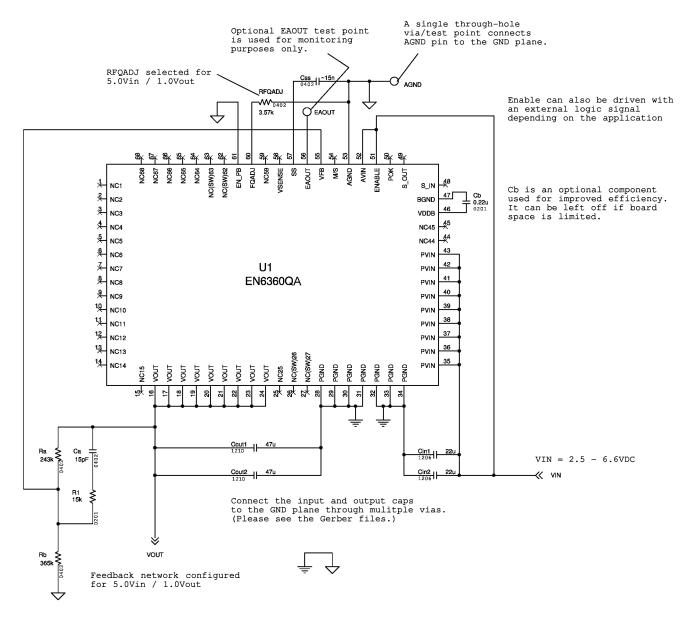
**Figure 9: Engineering Schematic with Engineering Notes**
