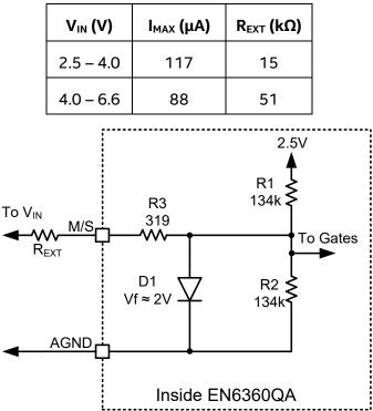
Figure 7: Selection of REXT to Connect M/S pin to VIN
