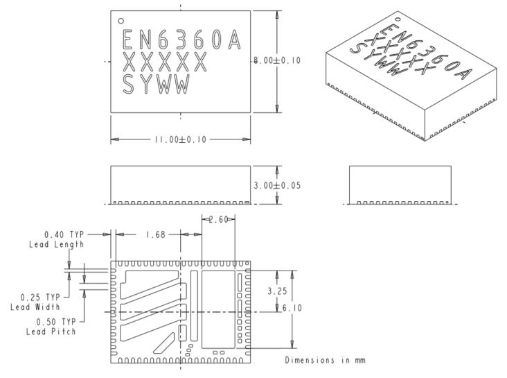
Figure 13: EN6360QA Package Dimensions (Bottom View)
