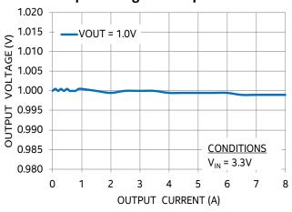
**Output Voltage vs. Output Current**
