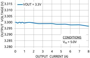
Output Voltage vs. Output Current
