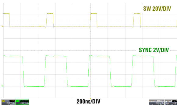
FIGURE 39. SYNC AT 1A LOAD, PWM
