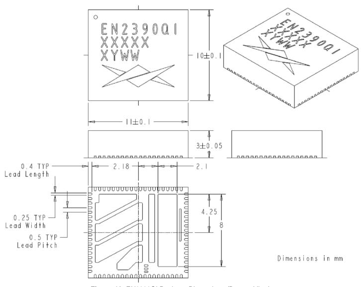
Figure 18: EN2390QI Package Dimensions (Bottom View)
