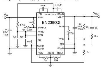
Figure 5: Single Input Supply Schematic
