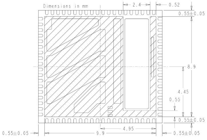
Figure 16: Lead-Frame exposed metal (Bottom View)
