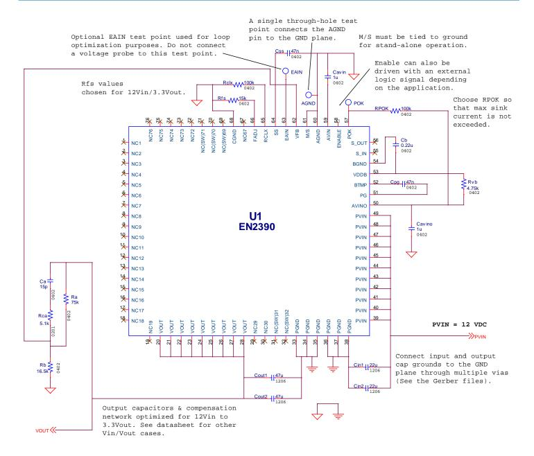
Figure 14: Engineering Schematic for Smallest Solution Size
