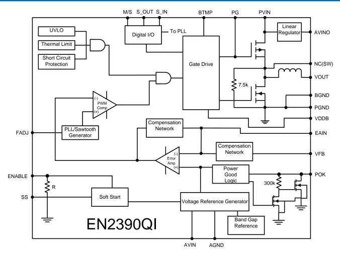
Figure 4: Functional Block Diagram
