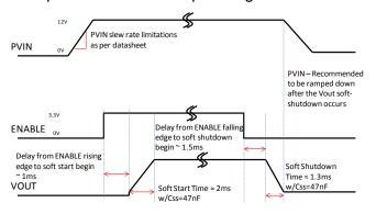
Figure 6: Single Supply Startup/Shutdown Sequence
