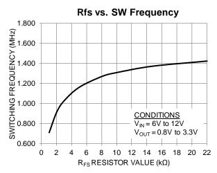
Figure 9. R<sub>FS</sub> versus Switching Frequency
