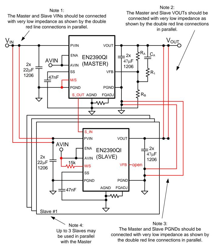
Figure 11. Parallel Operation Illustration
