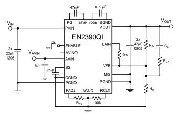
Figure 7: Dual Input Supply Schematic
