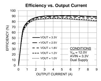
Figure 13: Efficiency vs. Output Current For  $V_{IN} = 12V$ ,  $V_{OUT} = 1.2V$  at 9A,  $\eta \approx 82\%$
