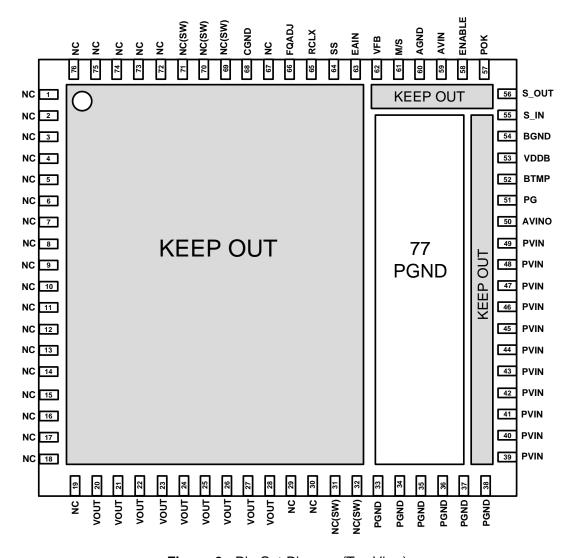
Figure 3: Pin Out Diagram (Top View)
