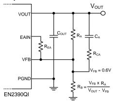
**Figure 12:** V<sub>OUT</sub> Resistor Divider & Compensation Components. See Table 4 for details.
