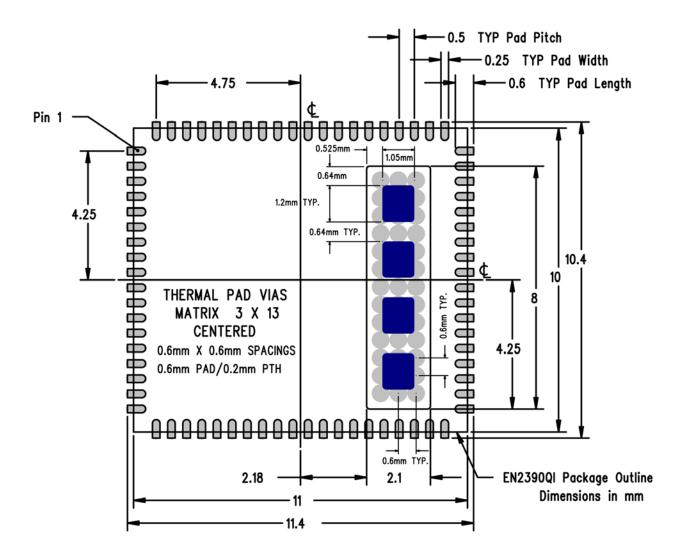
Figure 17: EN2390QI PCB Footprint (Top View)
