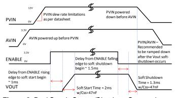
Figure 8: Dual Supply Startup/Shutdown Sequencing
