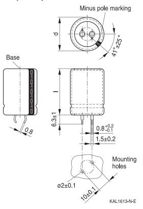
Snap-in terminals, length  $(6.3\pm1)$  mm. Also available in a shorter version with a length of (4.5-1) mm. PET insulation is marked with "PET" on the sleeve. Safety vent on the case wall.
