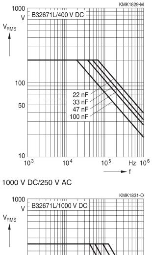
V = B32671L/1000 V DCMS 100 4.7 nF 8.2 nF 22 nF 10 10  $10^{3}$   $10^{4}$   $10^{5}$   $Hz 10^{6}$
