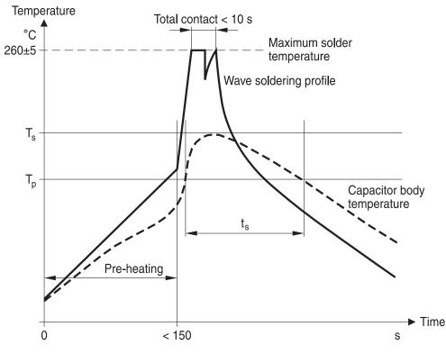
T<sub>s</sub>: Capacitor body maximum temperature at wave soldering T<sub>p</sub>: Capacitor body maximum temperature at pre-heating кмк1745-А-Е
