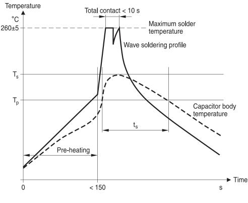
$T_s$ : Capacitor body maximum temperature at wave soldering  $T_p$ : Capacitor body maximum temperature at pre-heating
