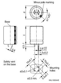
Snap-in capacitors are also available with 3 terminals (length (4.5 –1) mm). PET insulation is marked with label "PET" on the sleeve.
