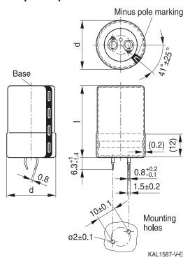
Snap-in terminals, length (6.3 + 1/-1.4) mm. Also available in a shorter version with a length of (4.5 - 1.4) mm. PET insulation cap is positioned under the insulation sleeve. Safety vent on the base.
