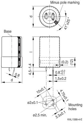
Snap-in capacitors are also available with 3 terminals (length (4.5-1.4) mm). PET insulation cap is positioned under the insulation sleeve. Safety vent on the base.
