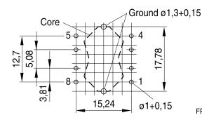
Hole arrangement View in mounting direction
