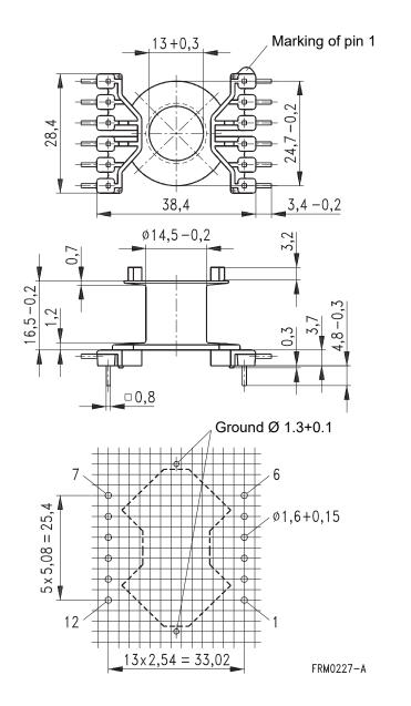
Hole arrangement View in mounting direction (Note half pitch!)
