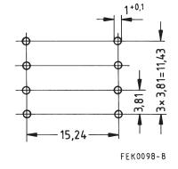
Hole arrangement View in mounting direction
