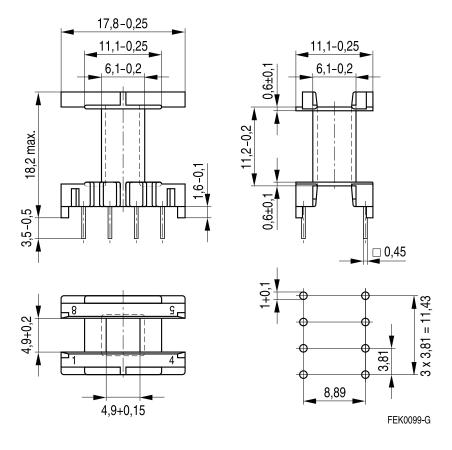
Hole arrangement View in mounting direction
