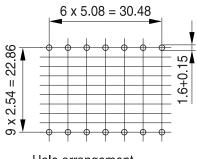
Hole arrangement View in mounting direction
