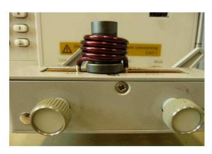
$2.9~\mu\text{H}$  The small distance between ferrite core and metal parts of measurment adapter causes a decrease of the measured inductance from 2.9 $\mu\text{H}$  to 2,7 $\mu\text{H}$ .
