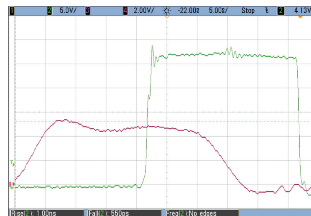
Figure 4: Typical Waveforms for V IN = 28 V to 3.3 V/4 A (5 MHz) Buck converter CH2: (V OUT ) Switch node voltage — CH4: V PWM Input voltage
