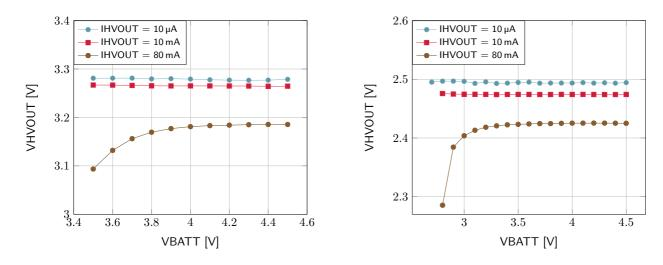
Figure 17: HVOUT at 3.3 V and 2.5 V
