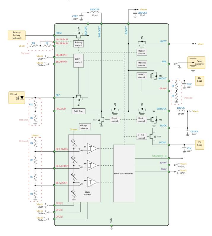
Figure 3: Functional block diagram
