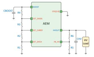
Figure 6: Custom configuration resistors
