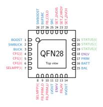
Figure 2: Pinout diagram QFN28
