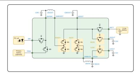
Figure 4: Simplified schematic view of the AEM10941
