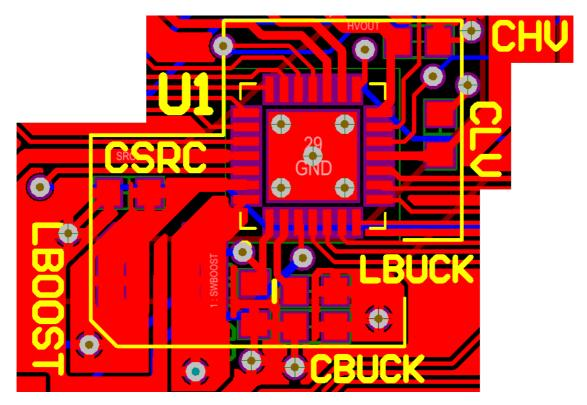
Figure 22: Layout example for the AEM10941 and its passive components
