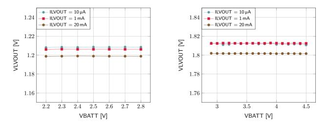
Figure 18: LVOUT at 1.2 V and 1.8 V
