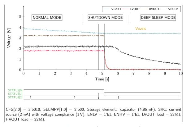
Figure 12: Shutdown mode (without primary battery)
