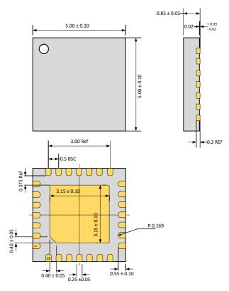
Figure 23: QFN28 5mm x 5mm
