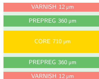
Figure 26: Recommended PCB stackup
