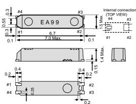
Do not connect #2 and #3 to external device. The metal case inside of the molding compound may be exposed on the top or bottom of this product. This purely cosmetic and does not have any effect on quality, reliability or electrical specs.
