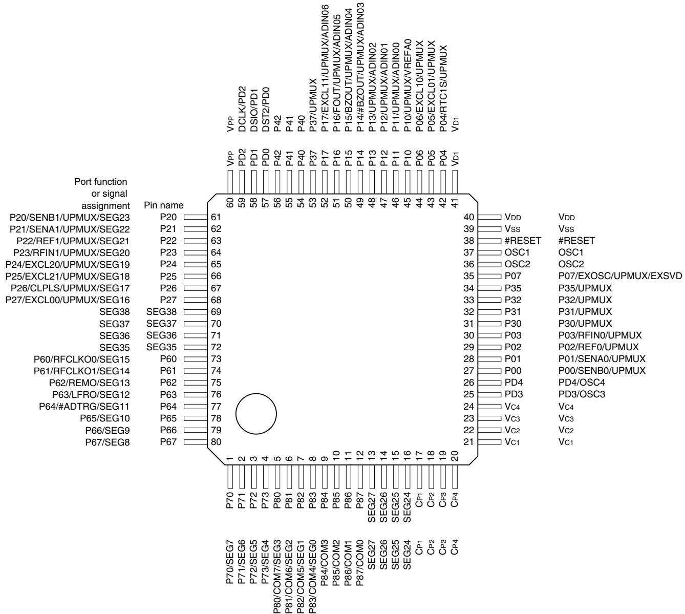
**Note:** The model in this package cannot be placed into super economy mode, as it does not have the V<sub>D2</sub>, C<sub>V1</sub>, and C<sub>V2</sub> pins.
