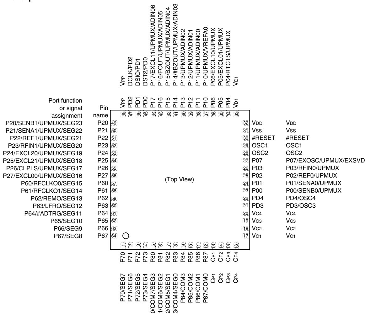
**Note:** The model in this package cannot be placed into super economy mode, as it does not have the V<sub>b2</sub>, C<sub>v1</sub>, and C<sub>v2</sub> pins.
