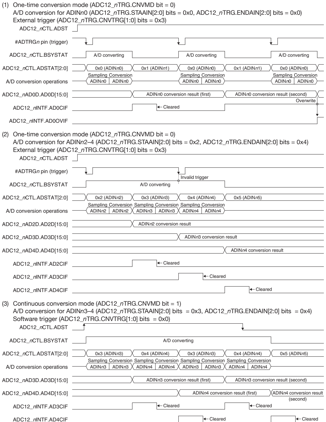
Figure 19.4.4.1 A/D Conversion Operations
