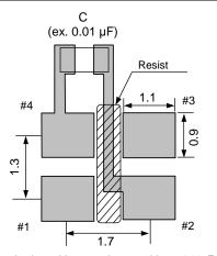
To maintain stable operation, provide a 0.01uF to 0.1uF by-pass capacitor at a location as near as possible to the power source terminal of the crystal product (between Vcc - GND).
