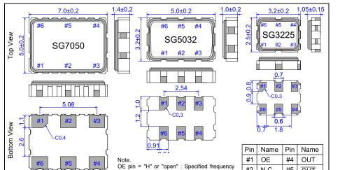
OE pin = "L" : Output is high impedance
