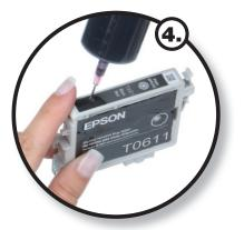
Now insert the syringe into the newly made opening and fill the ink chamber slowly and carefully until just below the opening. Should some of the ink leak out, simply remove it by using the syringe.
