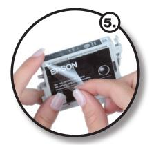
Seal the newly drilled hole with an adhesive strip and then leave the ink cartridge for a few hours to allow the ink enough time to spread throughout the ink chamber.
