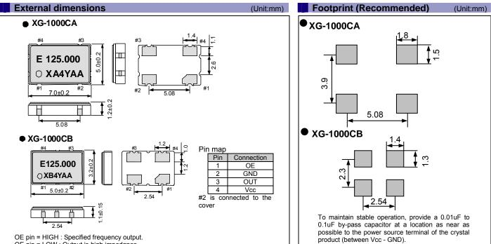
OE pin = LOW : Output is high impedance
