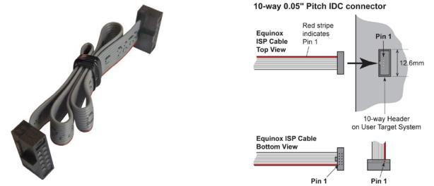
The **CAB-ARM-10W-150** is an In-System Programming (ISP) ribbon cable designed to connect from any ISP programmer which features a 10-way 0.05" pitch connector to a 10-way 0.05" pitch connector on a suitable ARM microcontroller Target System. The cable features 150 mm of flat ribbon cable with a 10-way 0.05" (1.27mm) pitch female connector on each end.
