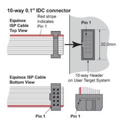
The **CAB-ISP10W200** is a **10-way** In-System Programming (ISP) ribbon cable designed to connect from any ISP programmer which features a 10-way IDC connector to a 10-way 0.1" pitch IDC connector on a suitable Target System. The cable features 200mm of flat ribbon cable with a 10-way IDC 0.1" pitch female connector on each end. The IDC connectors are fitted with 'cable grips' and are bump polarised to prevent the connector being plugged in the wrong way around.
