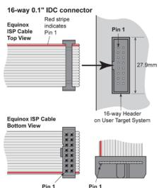
The **CAB-16W/16W-ISP-RIBBON** cable is a **16-way** In-System Programming (ISP) ribbon cable designed to connect from any ISP programmer which features a 16-way IDC connector to a 16-way 0.1" pitch IDC connector on a suitable Target System. The cable features 200mm of flat ribbon cable with a 16-way IDC 0.1" pitch female connector on each end. The IDC connectors are fitted with 'cable grips' and are bump polarised to prevent the connector being plugged in the wrong way around.
