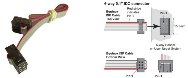
The **CAB-ISP6W200** is a **6-way** In-System Programming (ISP) ribbon cable designed to connect from any ISP programmer which features a 6-way IDC connector to a 6-way 0.1" pitch IDC connector on a suitable Target System. The cable features 200mm of flat ribbon cable with a 6-way IDC 0.1" pitch female connector on each end. The IDC connectors are fitted with 'cable grips' and are bump polarised to prevent the connector being plugged in the wrong way around.
