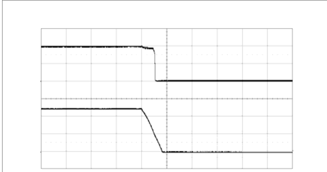
Shut-down enabled by disconnecting V_I at: T_{P1} = +25\text{ }^\circ\text{C} , V_I = 12\text{ V} , V_O = 1.0\text{ V} C_O = 470\text{ }\mu\text{F}/10\text{ m}\Omega , I_O = 40\text{ A} Top trace: output voltage (0.5 V/div.). Bottom trace: input voltage (5 V/div.). Time scale: (2 ms/div.).
