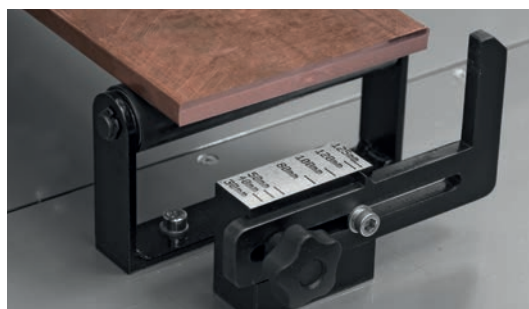
Additional busbars bumper, providing performance of perpendicular cut.
