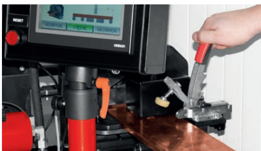
Holdfast for the busbars during cutting.
