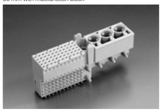
The ERmet type M female connector provides 55 contacts in a 5 row x 11 position (3 positions used by multifunction cavity), and also 3 contact positions for special power or coax contacts in a fully loaded configuration.
