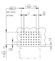
1) ø 0,6±0,05 Diameter of finished plated-through hole  $0.7 \pm 0.02 \ Diameter of drilled hole$
