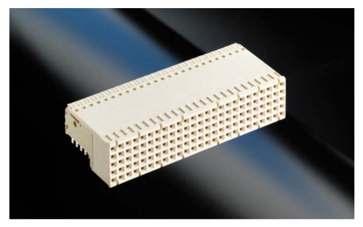
In the case of modern boards with SMT population, 2.0 mm H.M. ERmet thru hole reflow (THR) female connectors have been developed. The connectors have been designed for fully automatic SMT assembly. Safe positioning before the SMT soldering process is ensured by means of kinked terminations.
