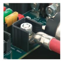
Attaching a cable to a M8 male thread PowerElement with twist protection (top left)
