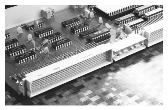
If extra connections are required on a standard double Eurocard, the Eurocard center connector can be mounted between the DIN 41612/IEC 60603-2 connectors. These connections can be used as signal contacts up to 4 A, high current contacts up to 40 A or coaxial contacts. Typical applications for coaxial contacts are:
