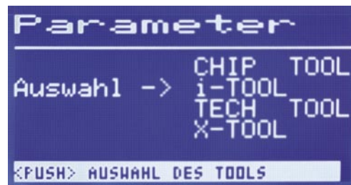
Tools are automatically detected when inserted into the station and a pre-determined program is started.
