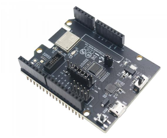
ESP32-C3-AWS-ExpressLink-DevKit with ESP32-C3-MINI-1 module
