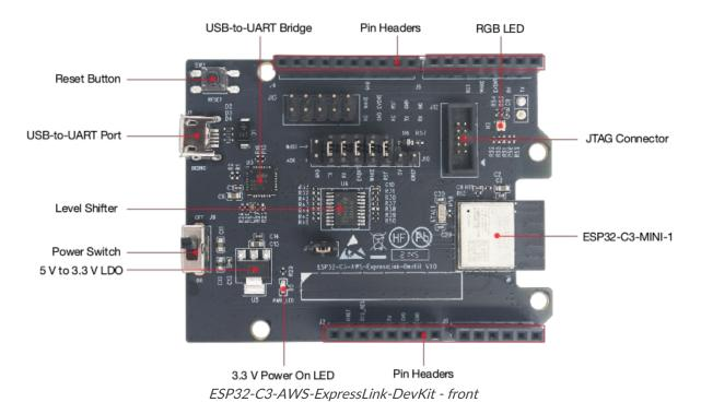
The key components of the board are described in a clockwise direction.
