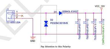
ESP32-C3-Lyra - Power Supply from 12V DC Input
